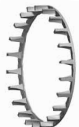
Fig. 46. Split, machined-brass, land-riding, finger-type cage.
