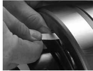
Fig. 91. Measure RIC before installation.
