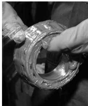
Fig. 147. Grease can easily be packed by hand.
