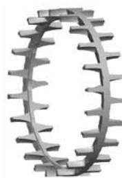
Fig. 44. One-piece, machined-brass, roller-riding, finger-type cage.
