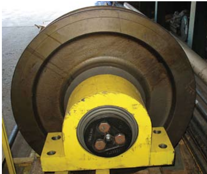
Fig. 12 AP bearings used in pillow block application
