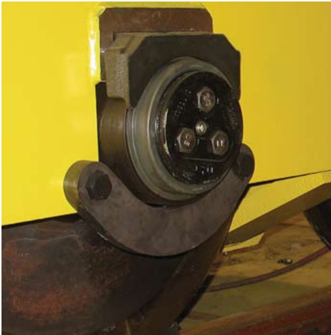
Fig. 8 Narrow adapter mounting on trolley safety bar
