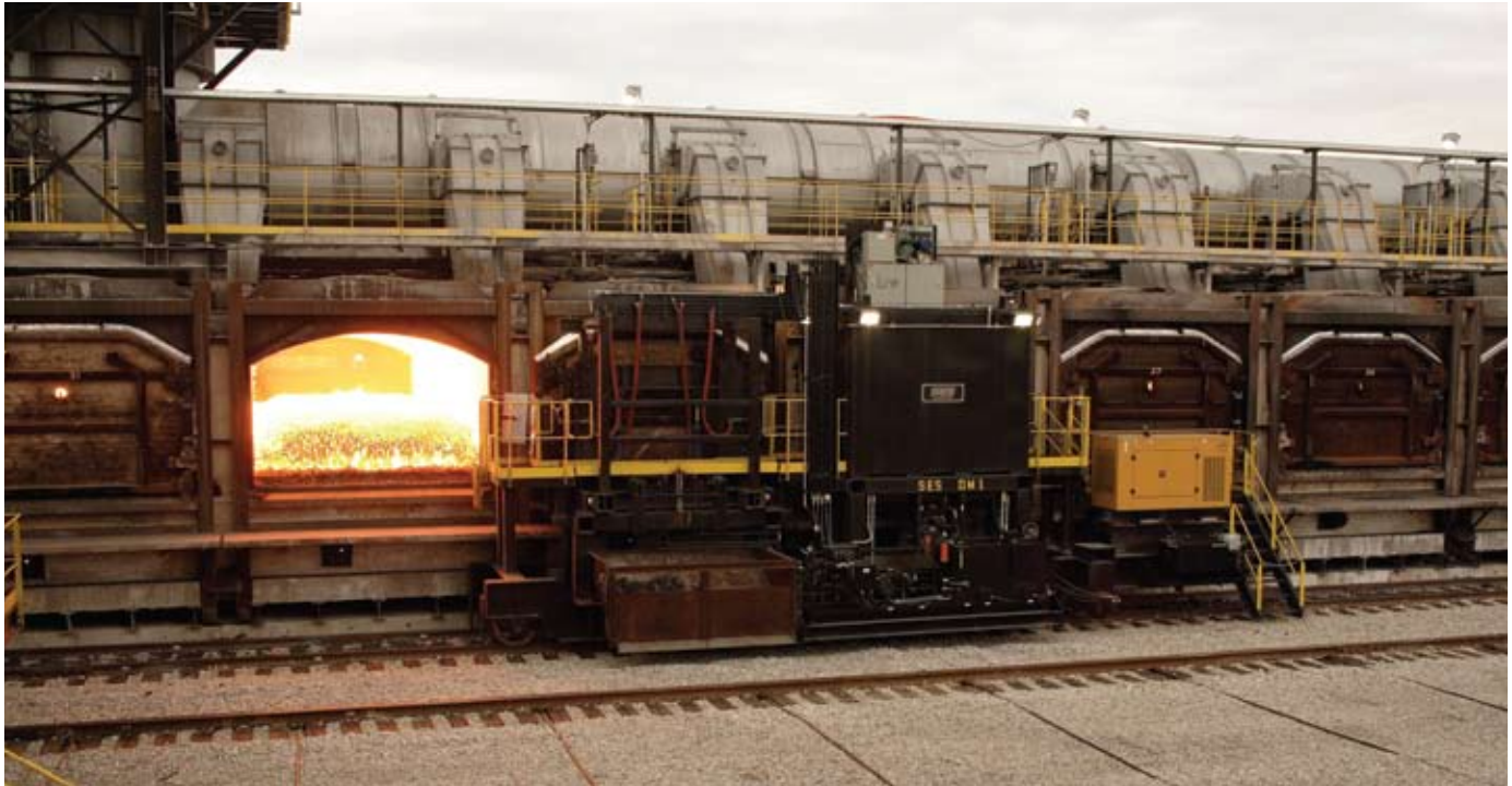
Fig. 20 Coke transfer car equipped with AP bearings
